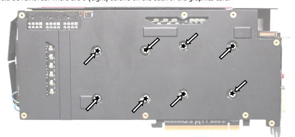
2.cont.: Remove the screws attaching the backplate to the circuit board. Remove the self-adhesive heatsinks from the circuit board as well! This step may require some force as adhesive might hold the heatsinks firmly to the PCB components. We recommend users to slowly and carefully pry the heatsinks from the PCB using bare hands (tool-less approach).
