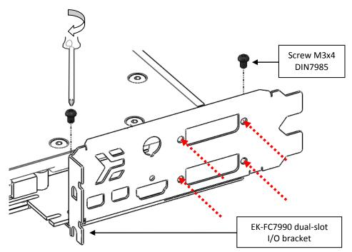
In order to move the 'Turbo' button from the original, three-slot I/O bracket to the EK provided two-slot I/O bracket take the following steps:
