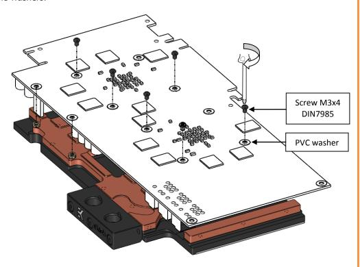
2. cont. By using enclosed Allen key 2mm screw in 4 (four) enclosed M3x9 DIN7991 screws. By using Philips head screwdriver secure the backplate using 2 (two) enclosed M3x4 DIN7985 screws.
