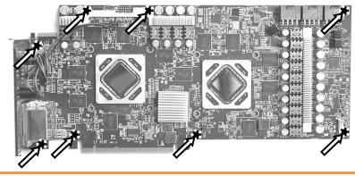
3. APPLYING THERMAL COMPOUND. Wipe off the remains (by using non–abrasive cloth or *qtip*) of the original thermal compound until the components and circuit board are completely clean. Apply thermal compound: lightly coat both *AMD* GPU chips as well as PLX bridge chip with - for example - GELID GC-Extreme<sup>™</sup> thermal grease. EKWB recommends to apply thermal grease in cross form for best performance (see sample picture).
