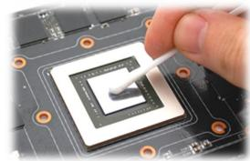
3. APPLYING THERMAL COMPOUND. Wipe off the remains (by using non–abrasive cloth or *q-tip*) of the original thermal compound until the components and circuit board are completely clean. Apply thermal
