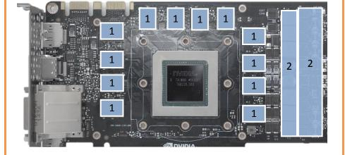
2. PLACING THE BLOCK ON TO THE GRAPHICS CARD. Carefully position the water block with preinstalled 2.5mm standoffs on to the graphics card. During this process please make sure you align mounting holes on the PCB with holes on the water block (same applies for other tops). Also pay attention not to use too much force by pressing the block down to the PCB. Chip dies are prone to cracking.
