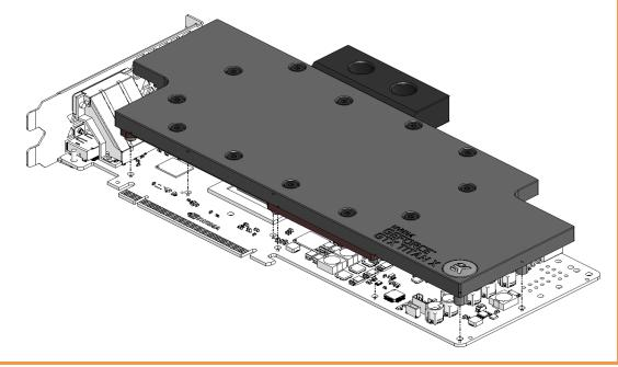
3. ATTACHING THE BLOCK TO THE GRAPHIC CARD. Use a Philips screwdriver with the enclosed M3x4 DIN 7985 screws. EKWB recommends users to start tightening the screws around the GPU core and continue outwards. To secure the I/O bracket please use enclosed M3x6 DIN 7985 screw.
