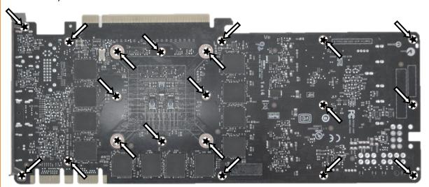
2. CLEANING THE PCB. Carefully detach the original stock cooler after removing **all** screws securing it to the board. Wipe off the remains (by using non–abrasive cloth or *q-tip*, as shown on sample photo) of the original thermal compound until the components and circuit board are completely clean. EKWB recommends the use of denatured alcohol for removing TIM leftovers.
